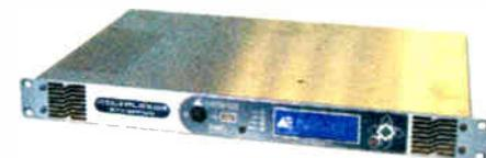
A choice of I/O termination panels with screw-terminal connectors makes connection easy. It is packaged in a 1RU enclosure and provides 64 digital I/O and 24 analog inputs, four serial ports, two Ethernet ports and four USB
