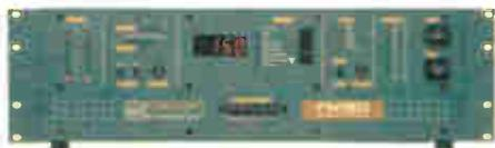
the FM600. Increased power output, front-panel frequency selection and increased remote control flexibility were incorporated in response to customer feedback. Existing models are upgradeable at nominal cost. A new color scheme will be applied across the Crown low-power FM transmitter line. Shipping is expected on July 1.
