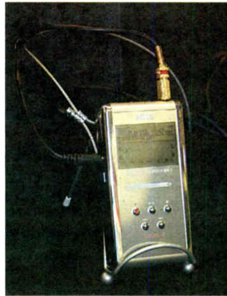
Korg announced a portable field recorder capable of recording up to 24-bit/192 kHz linear digital audio or audiophile-quality 1-bit, 2.8 MHz direct stream digital audio to its internal 20 GB hard drive, all in an iPod-sized package.
