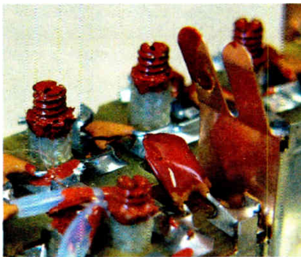
Fig. 1: The defective cap in this IF can is seen in the foreground.
