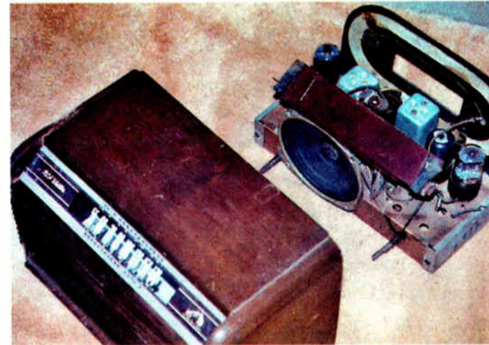
With a real wood cabinet, this RCA octal tube AA5 required a great deal of hand assembly. This particular one needs a new main tuning capacitor and restringing. Tubes included 35Z5, 12SA7, 12SK7, 12SQ7 and 50L6.
