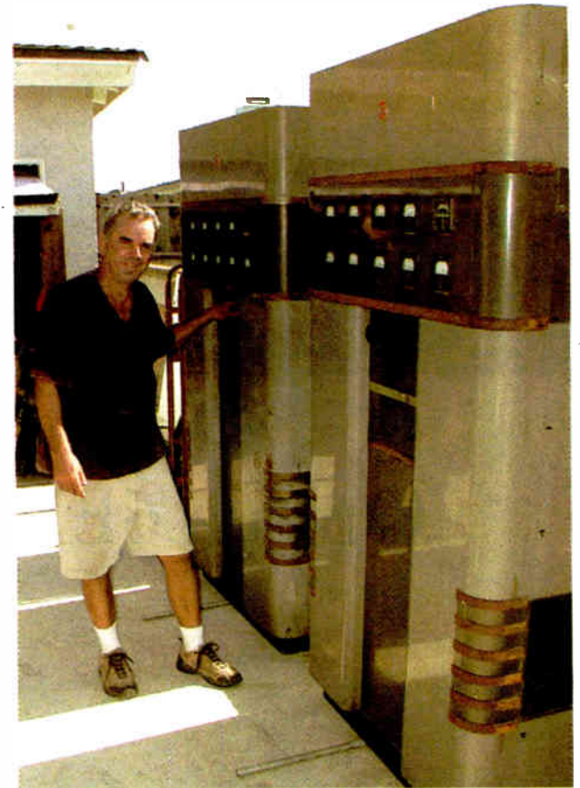
Horner and his Model 1-K, which consists of the Model 250-K transmitter and a matching amplifier unit.
