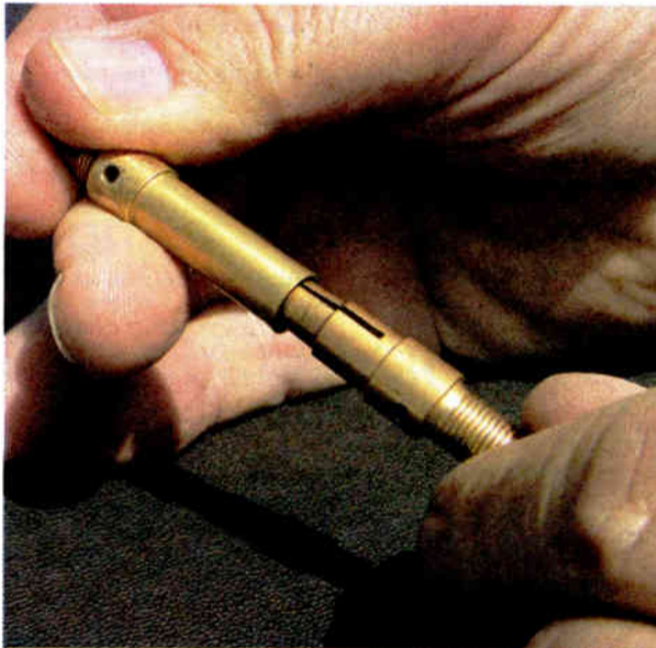
Fig. 1: Scrutinize used RF connectors before putting them to use.
