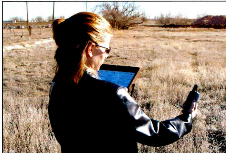
CBC-Denver Staff Engineer Amanda Alexander uses the GPS and FIM for a field strength measurement.
