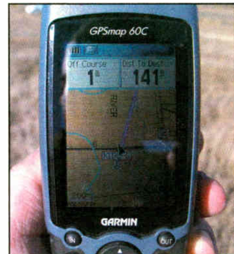
The Garmin GPS unit on a proof radial showing distance from the center of the radial and distance from the tower in meters.
