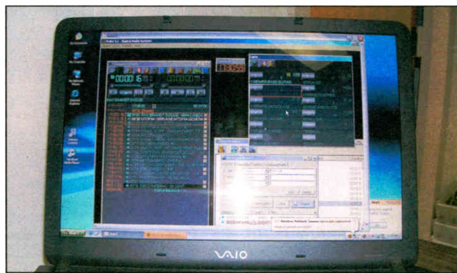
VNC software provides remote access to Dalet HD system at the main studio.
