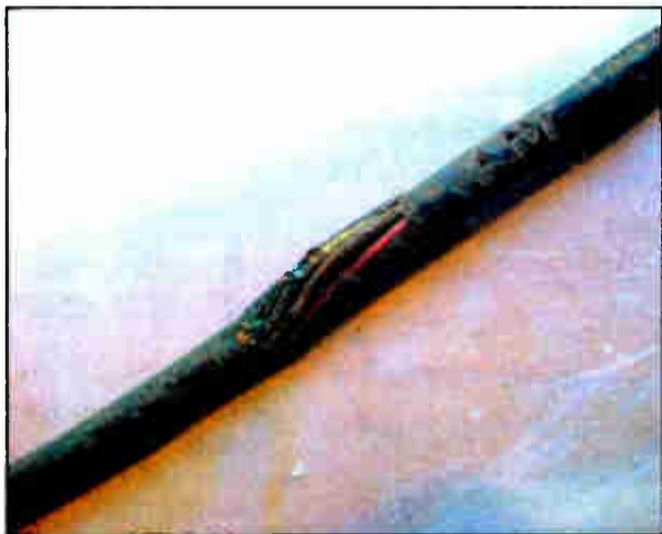
Yum! Fig. 1 shows the effect of rodents' sharp teeth on cable.
