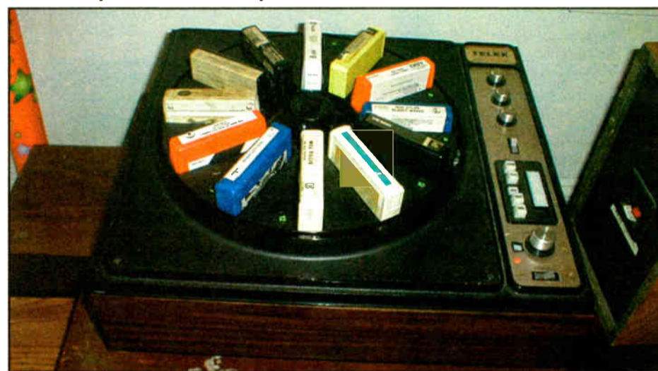
The Telex changer plays 12 8-track tapes back to back, for 8-9 hours of continuous music.
