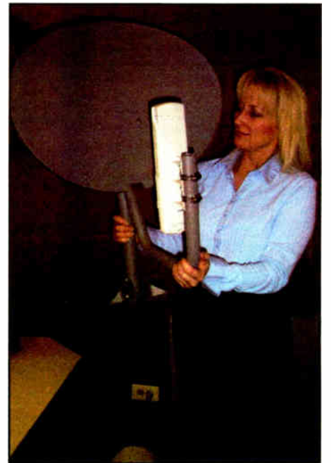
The Canopy helped Crawford solve a problem in Denver. The backhaul module with reflector is shown.
