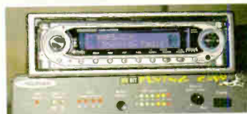
A Kenwood receiver displays the secondary digital channel, with the designation '2CH,' at the NPR Public Radio Engineering Conference.
