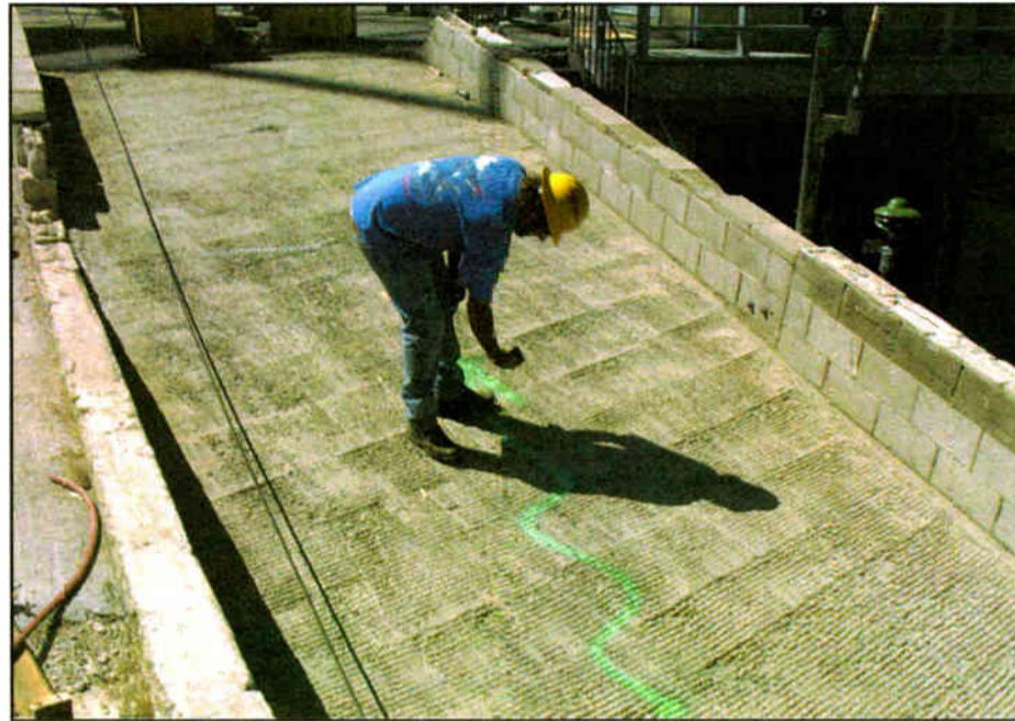
In a photo taken shortly after the original FCC inspection, a tower worker in the KMEX driveway uses a meter to measure a 'hot spot' marked by the commission with green paint.
