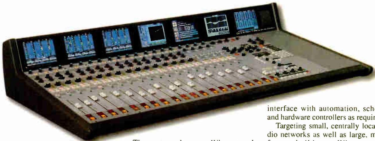
The system also uses Wheatstone's VDIP configuration software, so studio functions (like mutes, fader and timer starts, tallies, etc.) can be completed at a user's desktop. Once finished, settings are retained in non-volatile storage, allowing the system to run independently. Ethernet protocol is built in, providing
