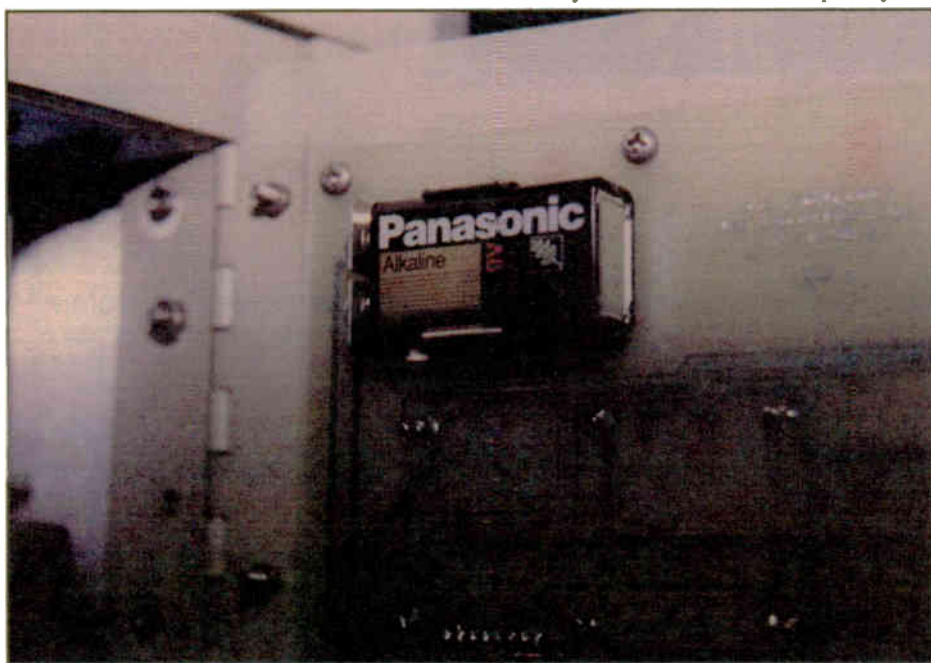
Fig. 1: Radio's secret power source? No, but if you don't replace the 'memory' battery in your transmitter on a regular basis, problems can result.
