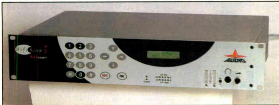
Features include an Ethernet interface so a station's codecs can be supervised remotely via a TCP/IP connection using Telescoop2 software running on a Windows system.
