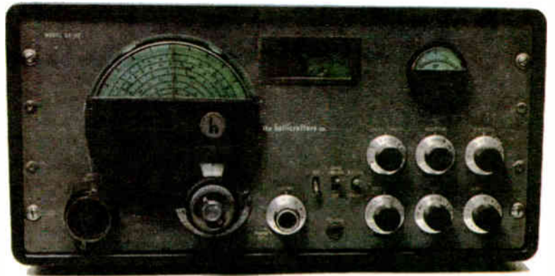
Nelson restored a classic Hallicrafters SX-42, a six-band receiver made in 1947.
