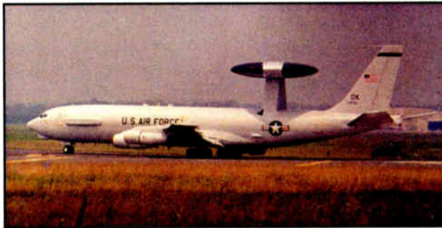
AWACs at work: The Air Force E-3 Airborne Warning and Control flying command post is distinguished by its rotating radome, which contains aerial surveillance radar. This one is at McGuire Air Force Base.
