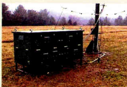
Model STM-AMAB-5K 5 kW All-Band Antenna Tuning Unit And Associated Telescopic Mast
