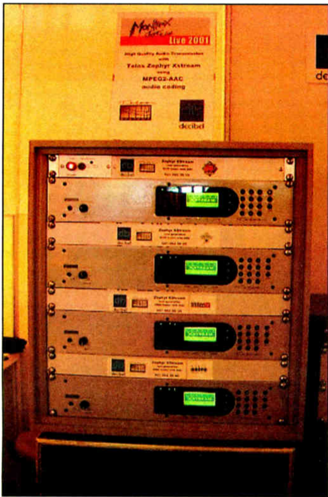
Telos Systems Zephyr Xstream codecs were in use at the Montreux Jazz Festival.
