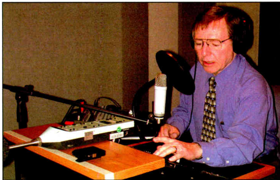
Jim Jensen, senior staff consultant at Arbitron's Research and Technology Center in Columbia, Md., conducts tests to ensure that codes placed in the audio stream of broadcasts cannot be heard by the human ear but can be detected by the PPM.
