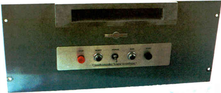
This ATC/Collins cart machine featured plug-in modules with vacuum tubes for both program and cue amps.
