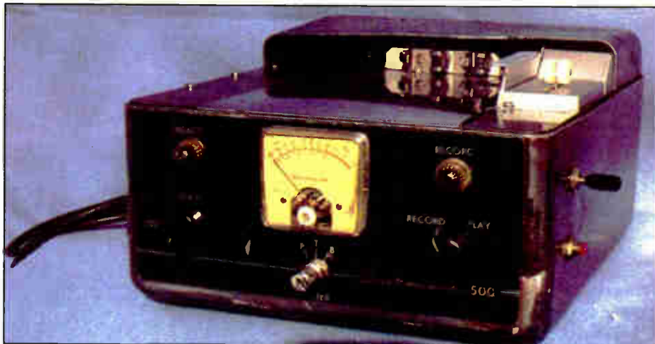
Shown is the first cart machine manufactured by Spotmaster. The original 500 contained both tube and transistor circuitry.
