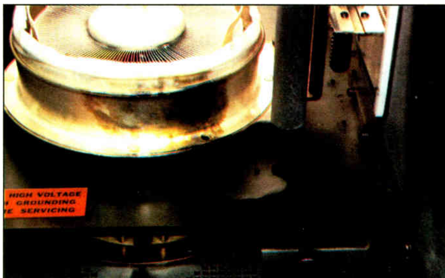
Figure 4: Misadjusted transmitter controls can literally cause a meltdown.
