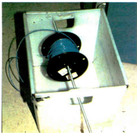
Figure 1: Here's a cheap way to manage wire.
