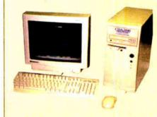
In a self-contained desktop system, the CDA 2000 provides simple test start and results screens. If a disc fails, the full digital analysis graphs and sector data printouts allows the engineer to isolate exactly where the error occurred.
