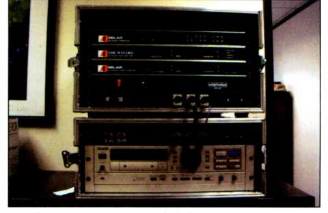
Packaged as two rack cases by Radio Systems, the Belar Wizard Mod Monitor and DAT for sample collection are a manageable set. Components can be used together or individually.
