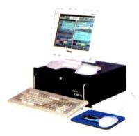
The ENCO  $DAD_{PRO}$  32 Digital Audio Delivery System provides a powerful professional audio management tool for both live assist and automated on-air operations, production, and inventory control. Support of Wide Area Networking is inherent with  $DAD_{PRO}$  32, providing capabilities to take full advantage of distributed data and group interconnectivity.
