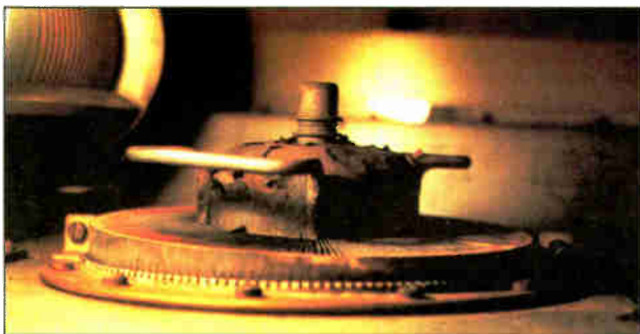
Figure 1: Tube life is quickly lost when a tube is starved for cooling air.
