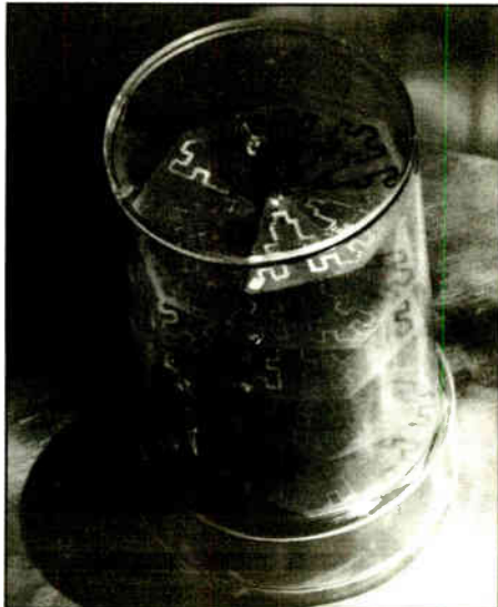
Figure 3: A fractal end-fire helix in a transparent radome attains the same gain as a regular helix three times its height. Shown here, a 675 MHz antenna measures 7.5 cm in diameter and about 12 cm high. Gain is about 7 dBi. A similar design for 450 MHz is 12 cm in diameter and 18 cm high.
