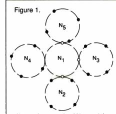
Above: An example of N-material with an extra electron added to the valence, or outer orbit, of atom N<sub>1</sub>.
