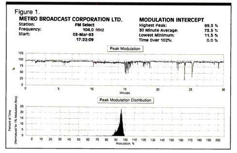
tive way to determine the gross overall amount of processing—or lack thereof—evident on your signal or on that of the competition. Unprocessed audio usually has a shallow, bell-curve distribution; modern processed audio has a relatively steep rise up to a peak just below the modulation limit, and then a sharp dropoff as it hits the limiting threshold.
