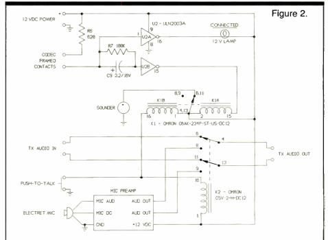
drives the inputs of U2A and U2B high. Driver U2A lights the "connected" indicator light to show that the system is in use. C9 differentiates the high at the input of U2B and sets latching relay K1, which beeps the piezo sounder. K1 may be any suitable dual-coil latching DIP relay. We used a Mallory SC616CP sounder, which features a chime tone, but other types are suitable.
