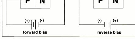
tion. Electrons line up on the P-side of the material and holes line up on the Nside
