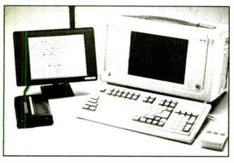
The STI-9000 incorporates state-of-the-art GPS and computing technology to provide a new method of analysis based on measured data. Contour plots quickly displayed by the STI-9000 simplify large amounts of data and improve visualization of signal parameters (antenna patterns, signal-to-noise ratio, bit error rate, etc.) over a measured area.
