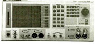
Panel settings can be saved in 99 internal memories, and also may be stored on an IC memory card, and for automated testing, full-function remote control is provided via GP-IB.
