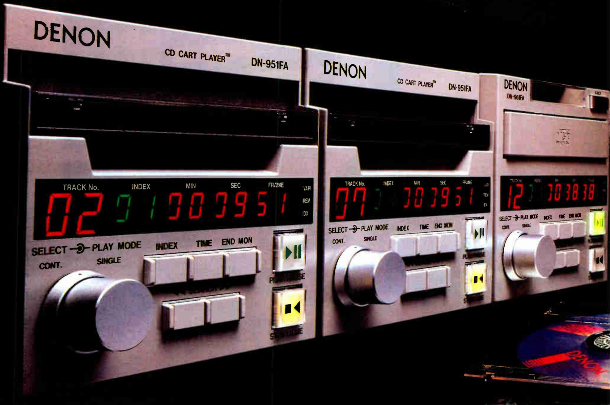
In broadcast circles, Denon CD Cart™ Players are the machines of choice. Now, broadcasters have an even greater choice—with the DN-951FA CD Cart™ and its Auto Track Select (ATS) system. This intelligent design reads bar-coded carts (easy-to-program ACD-5B cartridges) to lock-in, lock-out or auto-cue to a specific track.
