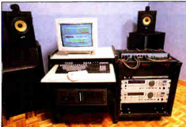
The SADiE system is a low-cost, IBM-platform audio editor with a user-friendly edit display.
