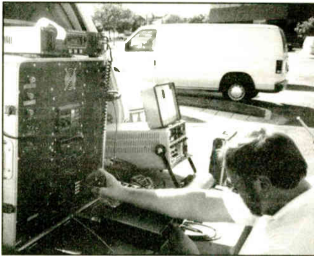
TFT's Terry Peterson sets up EIS for a remote-transmission trial in heavy multipath conditions. The Sage and ISL systems were earlier put through the same test.
