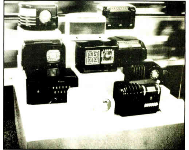
The use of plastic in radios became popular after World War II, ushering in an era of curved design.
