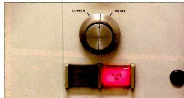
Scott’s LED fix for the push button switches.
