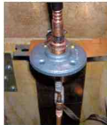
A custom-built 7/8" adapter.
