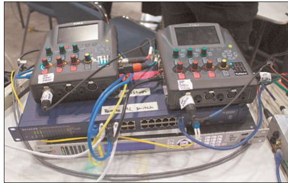
ViA codecs feeding main program audio for both shows with Merlin for backup.
