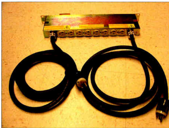
Back side of the Pulizzi transfer switch. One plug goes into the UPS output, the other into Mains (or a second UPS). The eight outlets feed critical or finicky equipment.
