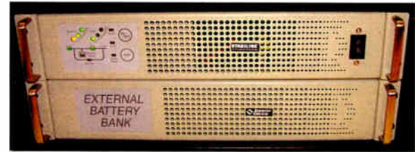
A true UPS with an external battery.
