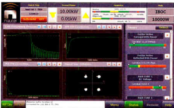
The AUI monitors the load and pre-correction data.
