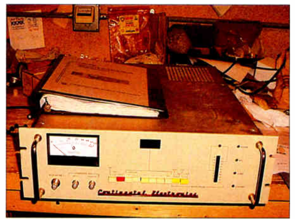
A frequency-agile exciter makes a simple emergency exciter or transmitter.
