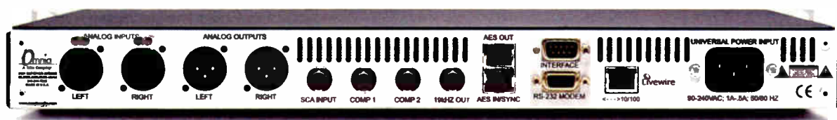
The rear of the Omnia ONE.
