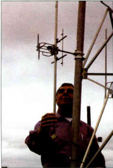
Using scale models, Shively can quickly test the effects of various antenna mounting solutions.
