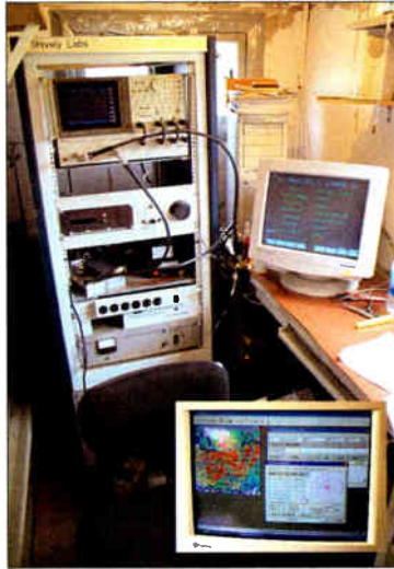
By measuring the radiated pattern of an antenna, the range technician can ensure it can be mounted in the best location to cover a station's market area.
