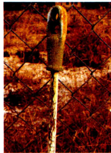
The surface of this fiberglass insulator was broken down allowing moisture and carbon tracks to form in the frayed surface.
