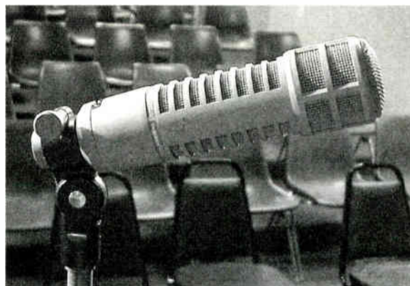
The ports on the side of an ElectroVoice RE20 affect polar response.
