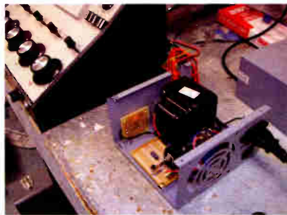
The repurposed power supply connected to the console. The existing case had the AC socket and on/off switch already in place.
