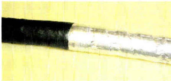
Heat Resistant Mastic Overlaps Foil
