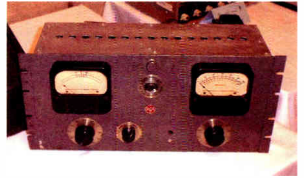
An RCA Model BW66E Modulation Monitor
