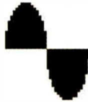
The original signal presented to an analog-to-digital converter.
