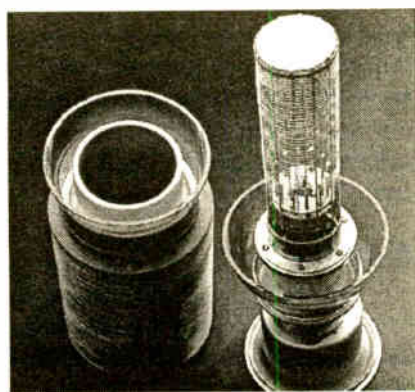
Tube Opened on Glass Lathe
