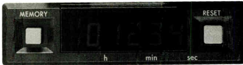
Tape accurate at all speeds, a microprocessor-controlled real-time counter features a Memory Rewind and L.E.D. display in hours, minutes and seconds.
