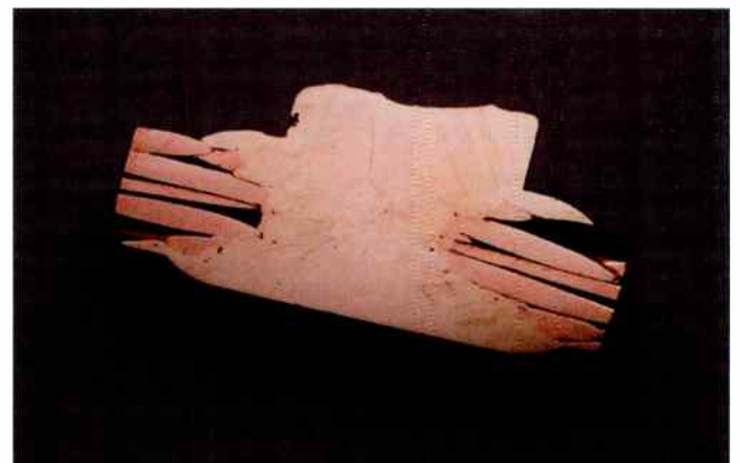
Photo 3. A cross section of an exothermic weld shows how it combines metal between a stranded conductor and a solid conductor. These welds work with a wide range of materials and shapes of conductors.
