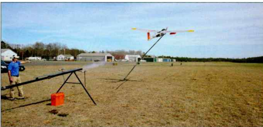
Shown as it was being launched, the RS-20 drone used in the test of airborne LTE conducted in Woodbine, New Jersey, carried equipment to connect it wirelessly with the Verizon network core. The 165-pound drone has a 17-foot wingspan.
