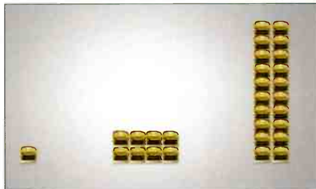
The capability of the 2-watt RF output base station cube is scaled up by using more of them in a combination, instead of making the individual base station cube bigger. For example, 20 could be placed in columns of 10 each inside a radome to form a multicarrier base station-antenna combination on an existing tower.
