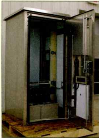
WiMAX Enclosure DDB Unlimited's outdoor WiMAX enclosure model OOD-54DX-GP-42 is designed for both large-scale build-outs and single-cabinet applications. Constructed of 0.125-inch-thick aluminum, the cabinet can be pad-, pole- or wall-mounted. Thermal options include 4,000-Btu air conditioning or direct-air cooling. www.ddbunlimited.com
