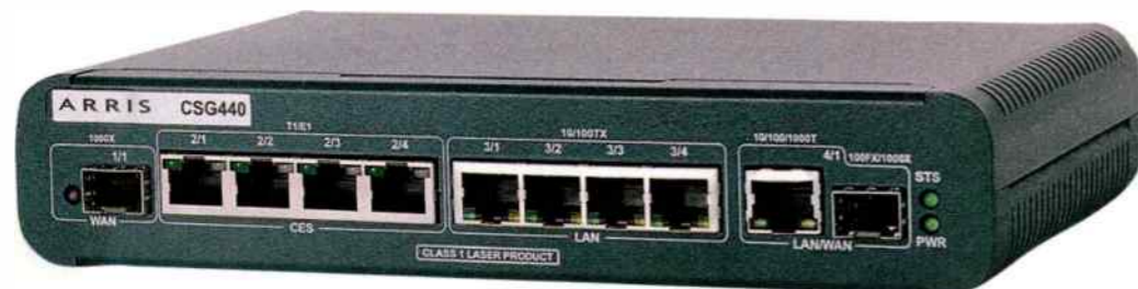
The Commercial Services Gateway (CSG440) by Arris provides Fast (nominal 100 Mbps) and Gigabit (nominal 1 Gbps) Ethernet demarcation gateways with T1/E1 circuit emulation services connectivity over Ethernet/IP Fiber networks.
