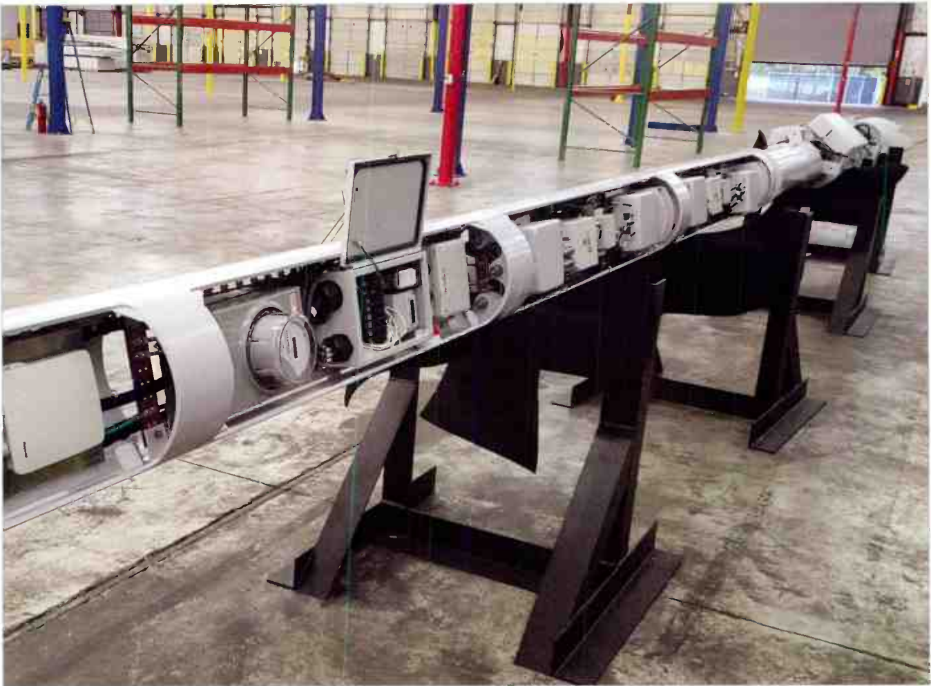
Photo 1. A typical AC power and equipment compartment in an integrated 5G small cell pole.
