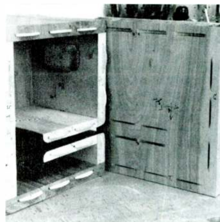
PHOTO 8: Preparing for the final side gluing. The large number of biscuits must be glued simultaneously.
