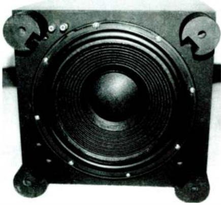
PHOTO 7: DV-12. Note rubber surround, stair-railing feet, aperiodic holes, and binding posts.
