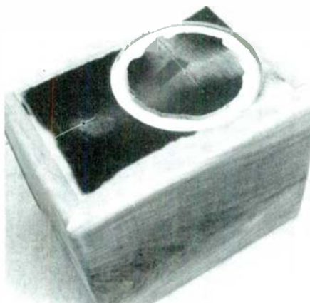
PHOTO 10: The results of the first step in routing the mid-range driver hole.
