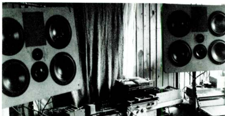
PHOTO 2: Coaxial dipoles. Note position out in room, with sound absorption. Behind open 1" x 4" wall is bass trap.
