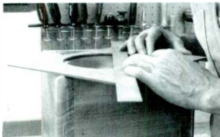
PHOTO 9: Aligning the template to cut the hole for the mid-range driver.
