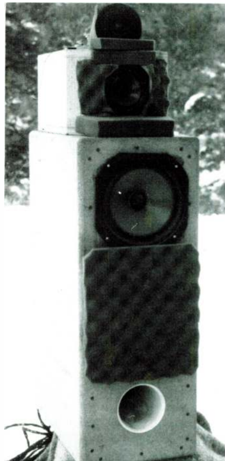
PHOTO 5: Monopoles. Note the offset and the foam.
