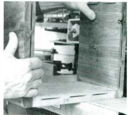
PHOTO 5: Sanding edges flush before going to the next step.
