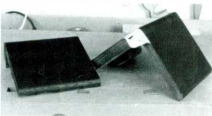
PHOTO 2: Paint the surfaces that would be impossible to reach after assembly. Note the use of masking tape to keep paint off the glue-joint surface.
