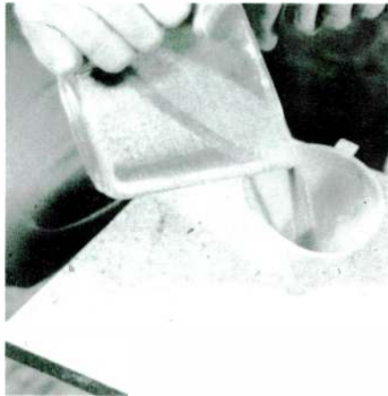
PHOTO 9: Filling the column with sand.
