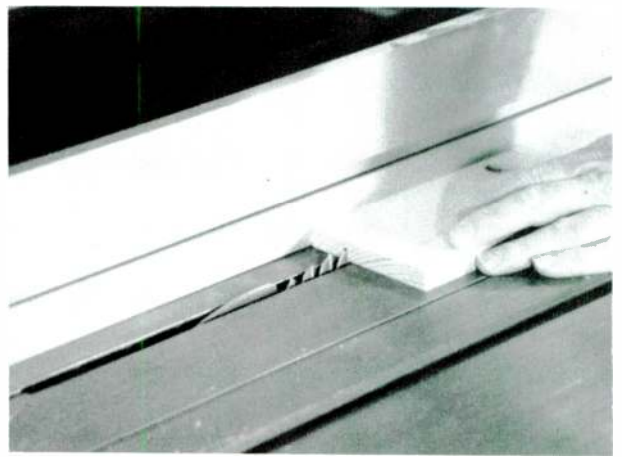
PHOTO 12: Cutting the first part of the groove for the sides of the top box.
