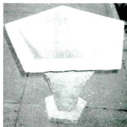
PHOTO 11: The horn's inside finished with Hammerite.
