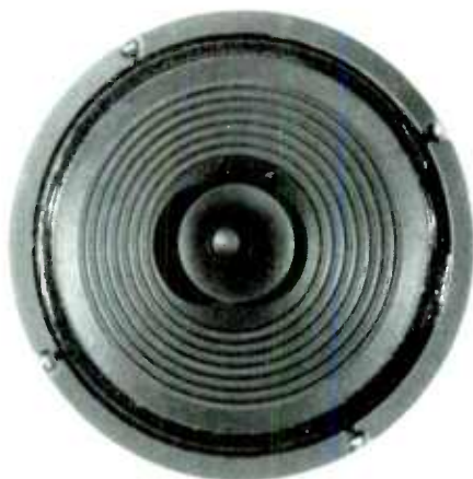
PHOTO 17: Speaker mounted in the board. Note how closely the speaker fits into the hole. This set of cuts was made on particleboard; MDF produces even better results.
