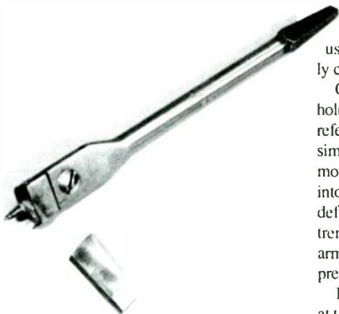
PHOTO 3: Expansion bits for use with a brace. The maximum radius is limited, usually to less than 2".
