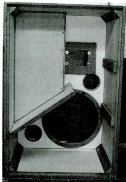
PHOTO 3: Midbass enclosure within main box.
