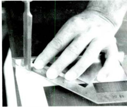
PHOTO 17: Marking the other end of an inlay strip. Remove the strip and cut off the excess, as shown in Photo 16 .
