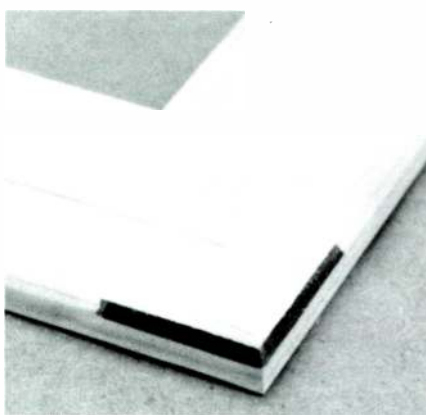
PHOTO 13: Soft-to-hard edge, made by lowering the roundover router bit so the upper edge cuts into the frame.
