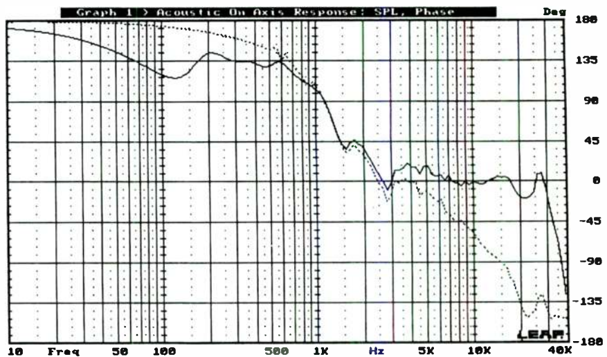
FIGURE 3: Comparison of measured phase (MLSSA) and calculated phase (LMS) for tweeter response of system depicted in Fig. 2.
