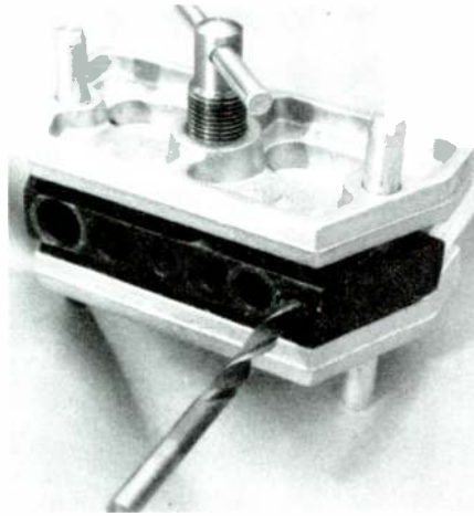
PHOTO 1: Using the Dowel-It jig for reinforcing the grille frame.
