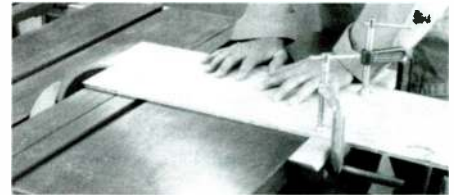
PHOTO 2: Technique for sawing large panels.
