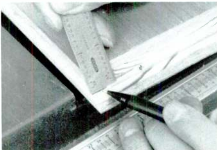
PHOTO 6: Marking the reference distance of 1/16" down from the inside edge of the joint. (The mark has been darkened to make it visible in the photo.)
