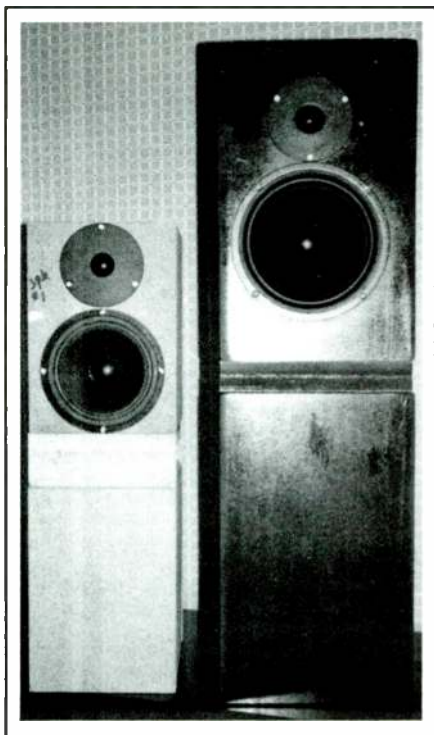
PHOTO 1: The 5" Vifa 3/4" Vifa speaker on the left, 6 1/2" Vifa 3/4" Scan Speak speaker on the right.
