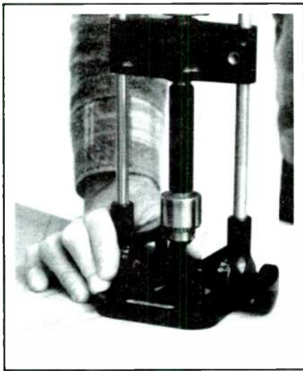
PHOTO 1: Drilling holes in side panels.
